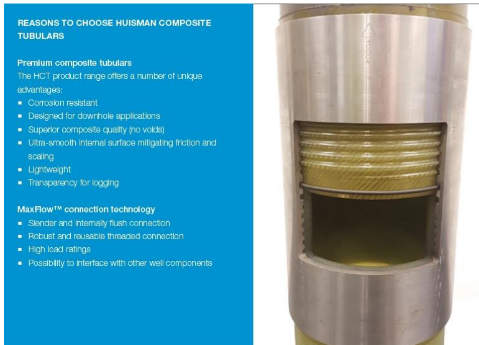
Figure 12. Example of GRE connection suitable for downhole applications. Source Huisman Geo.
