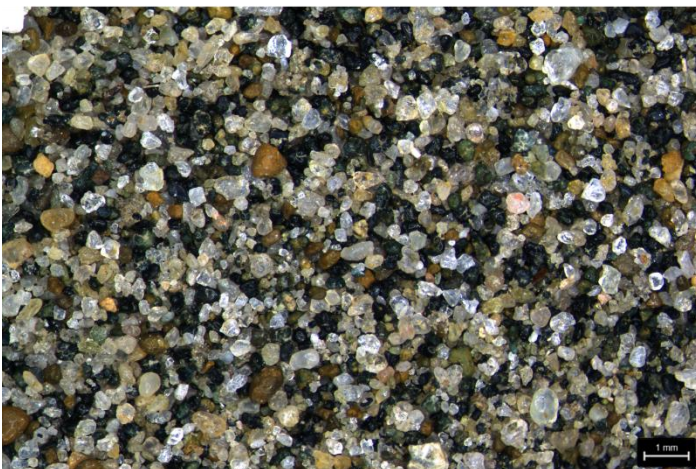
Figure 3-1: a) Sample from HVB-01, 220-230m MD. b) Microscopic image of the sample. c) Binary image with only the glauconite grains selected based on their colour.
