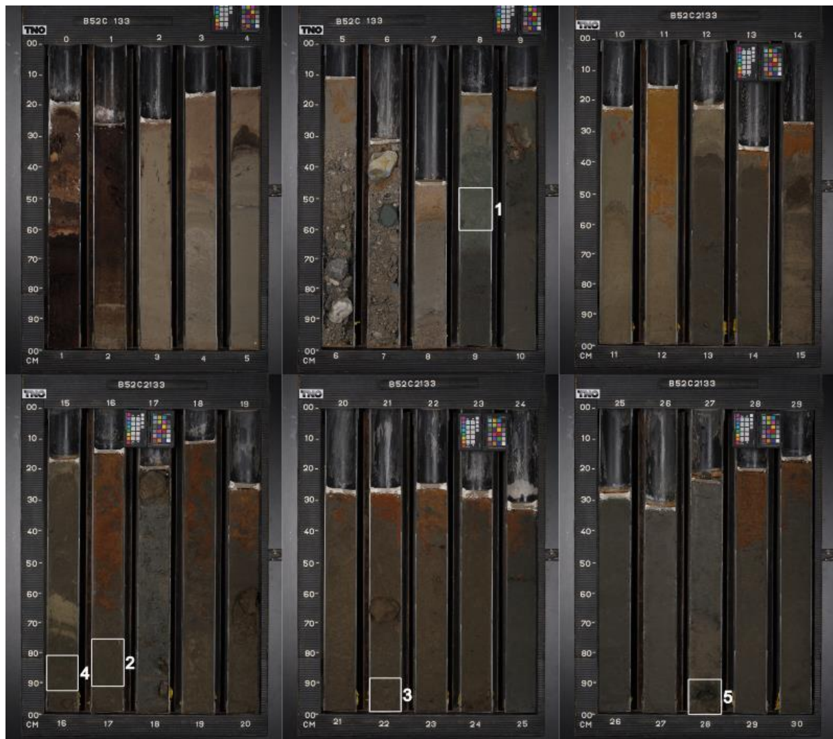
Fig. 2.5 The sawn out sample locations of samples 1-5 (white boxes) in an overview of core B52C2133 located in Liessel (Fig. 2.3). Sample 1: 847-860 cm (box 1); sample 2: 1675-1691 cm (box 2); sample 3: 2188-2200 cm (box 3); sample 4: 1582-1593 cm (box 4); sample 5: 2789-2800 cm (box 5). The top of the core is visualized by the upper left image and the bottom by the lower right image. Reddish parts contain more iron.
