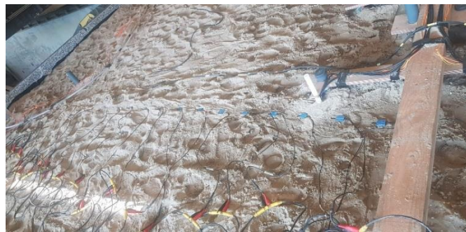
Figure B11: Geophone array to obtain reference V_p inside the partially saturated sand layering.
