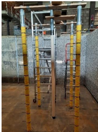
Figure A9: a) ERT array along 4 survey poles, and b) 4-poles array including injection (within the ERT array) and extraction (at the right end) wells.
