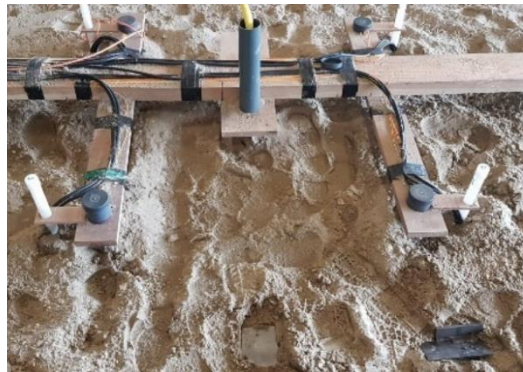
Figure A8. a) Overview of the test site with the DAS array, the injection and extraction wells, and b) Top view of 4-pole array for the cross-hole test.
