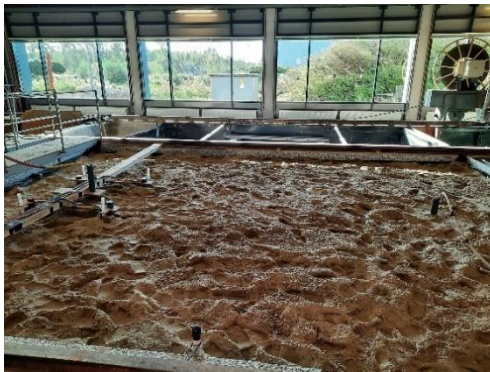
Figure A8. a) Overview of the test site with the DAS array, the injection and extraction wells, and b) Top view of 4-pole array for the cross-hole test.
