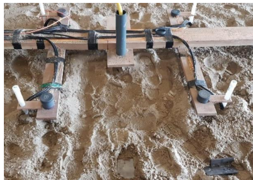
Figure B8 a) Overview of the test site with the DAS array, the injection and extraction wells, and b) Top view of 4-pole array for cross-hole test.
