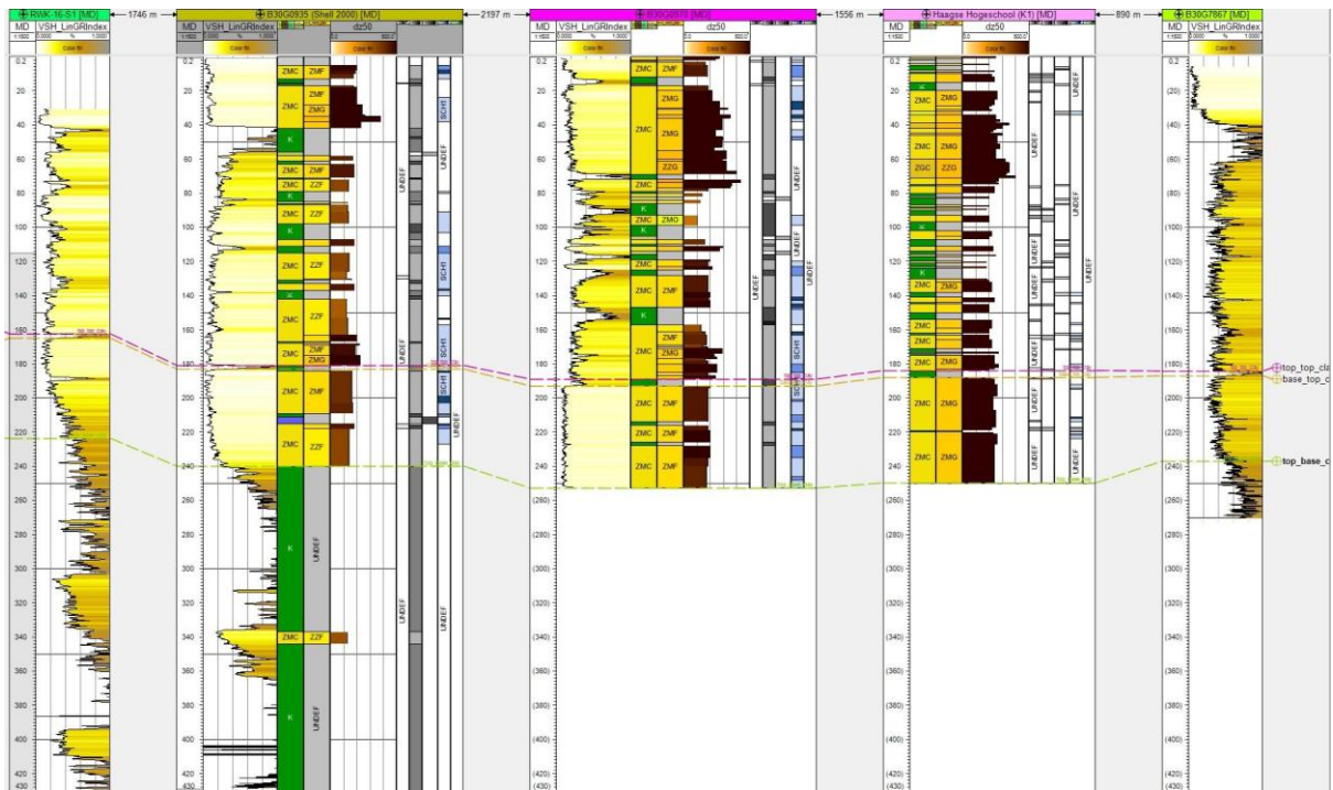
Figure 7 Well panel from south to north showing from left to right the RWK-16 O&G well (GR only), two shallow wells with lithology descriptions and GR log, the ATEs well ‘Haagse Hogeschool’ having a lithology description only and a shallow well with GR-log only. The tracks show GR, scaled GR, lithology, sand grain class and size, clay, silt and sand fractions, and shell content. Interpreted horizons are the top and bottom of the top sealing clay, and the base of the aquifer where applicable. Well locations on Figure 3.
